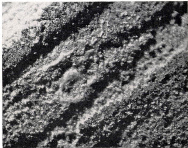
Fig. 5. Photograph of an etched electrode surface.
